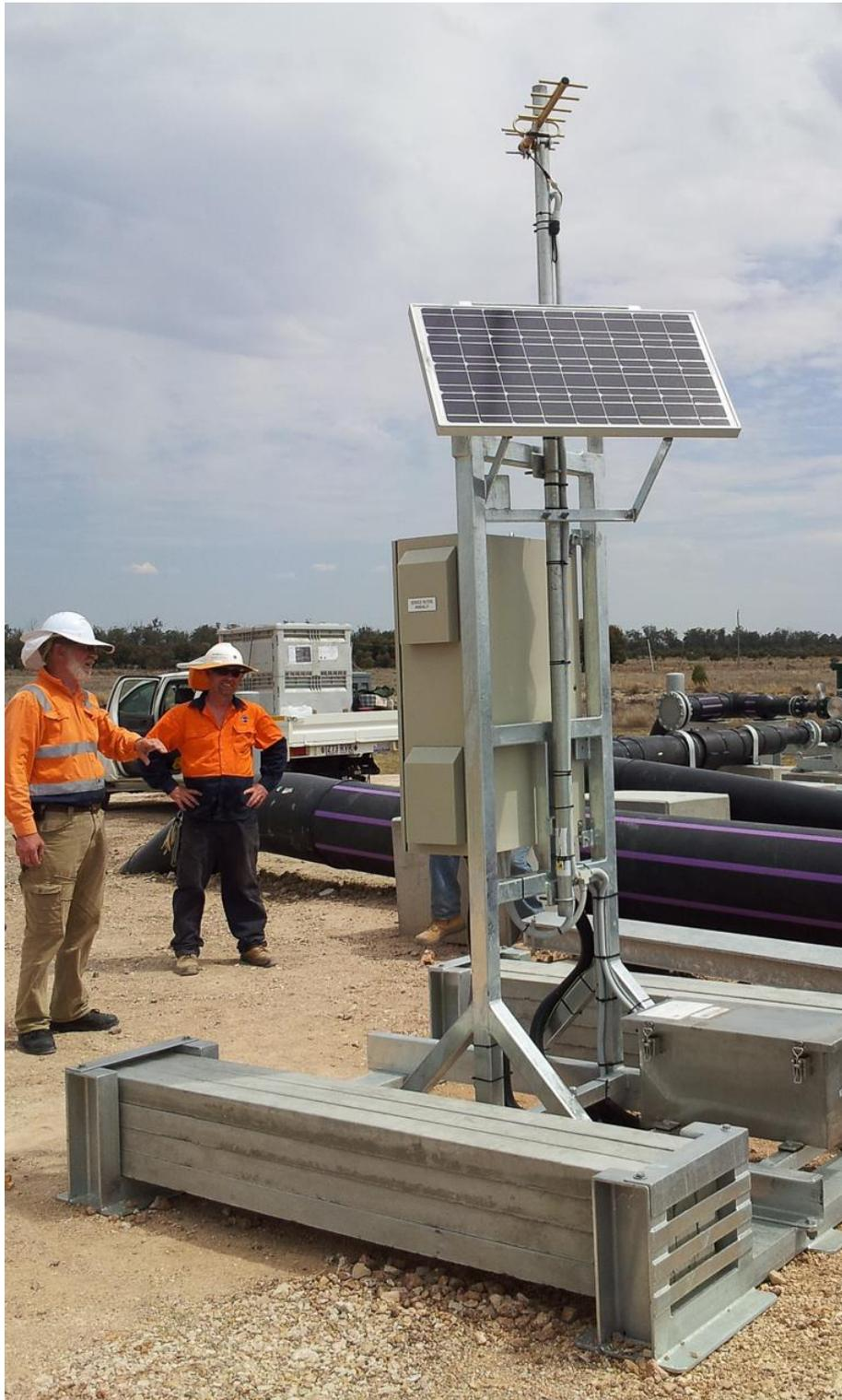
The device also measures pond telemetry including temperature, depth and salinity. Systems can be installed at the time of pond construction or retrofitted to an existing pond.
