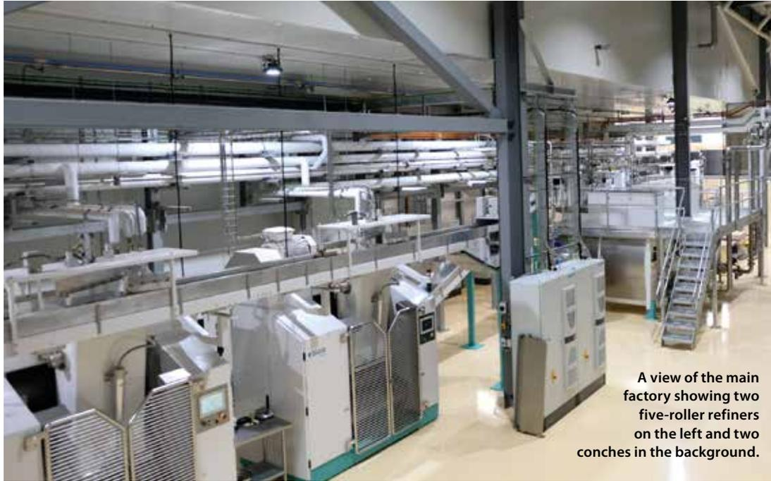
A view of the main factory showing two five-roller refiners on the left and two conches in the background.
