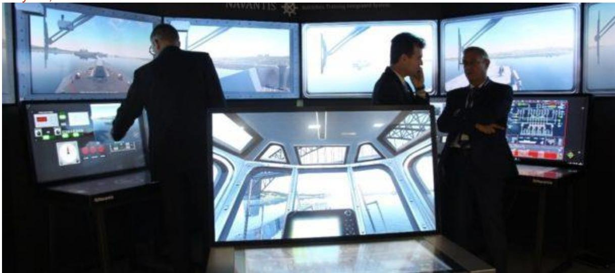
*Navantia's integrated training system Navantis on display at the PACIFIC 2017 summit. Navantis is a combined IPMS and navigation virtual simulator providing 2D and 3D IPMS views and interconnects with different ship simulators to allow simultaneous training of ship crews.*
