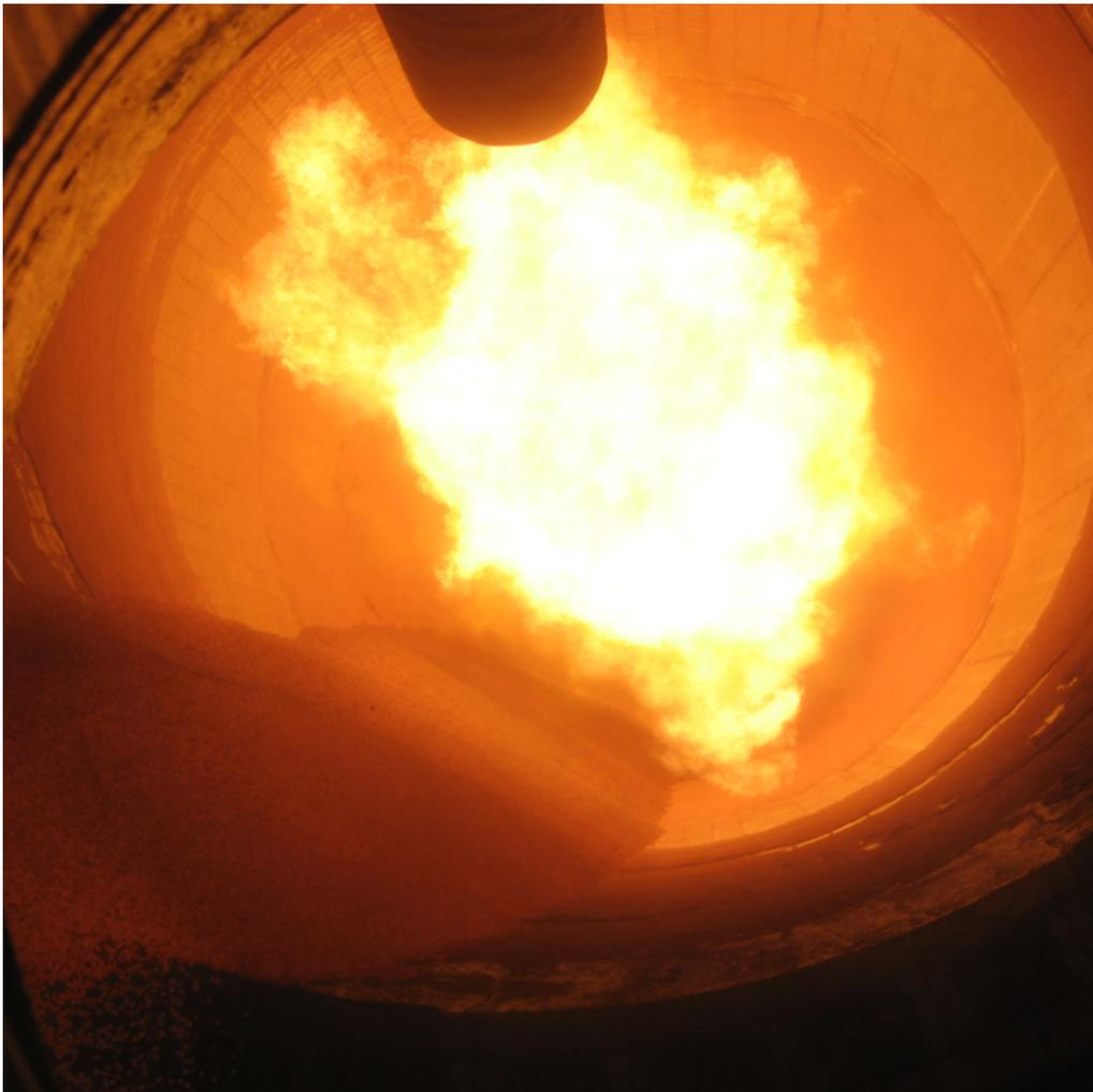
An FCT burner in action at an iron ore pelletizing plant.
