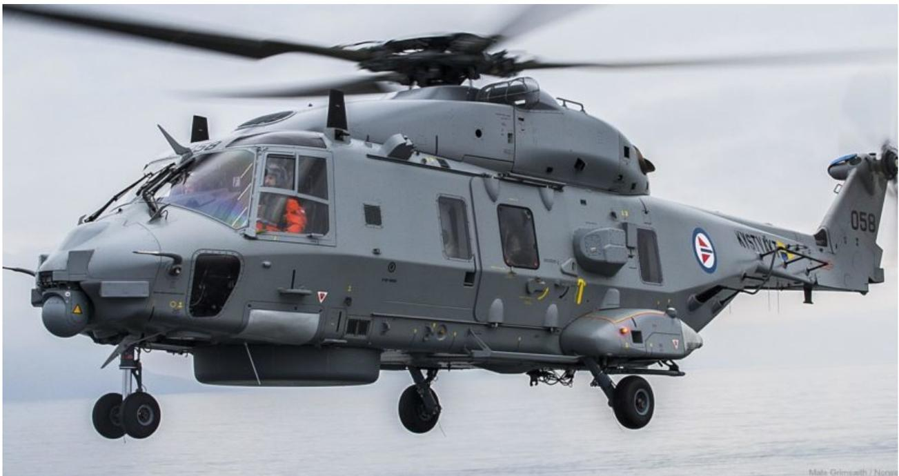
The NH90 is a medium-sized, twin-engine, multi-role military helicopter, developed in response to NATO requirements for a multiple capability helicopter. Photo: supplied
