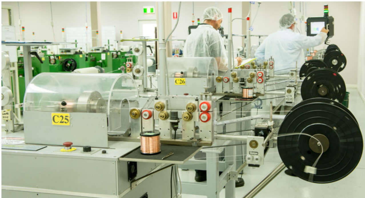
Several of the new machines built by Key Tubing & Electrical to produce the copper heater cable. Picture: Iain Bond
